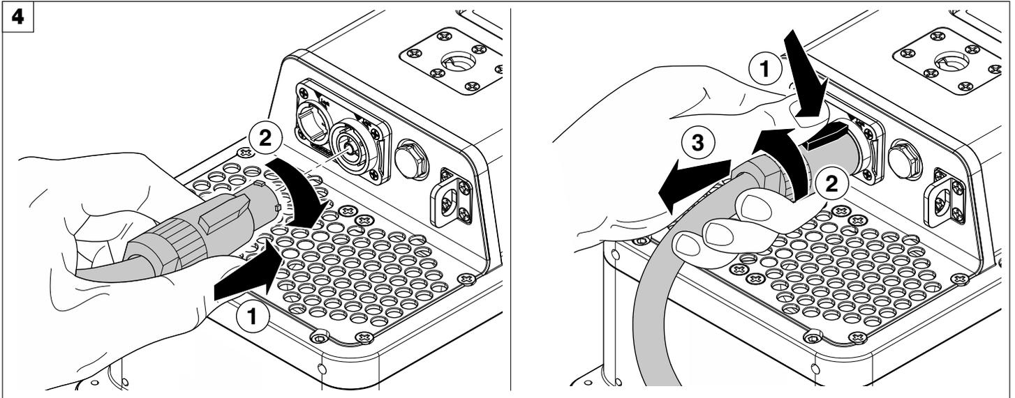
Connecting and disconnecting the power cord - Fig. 4
